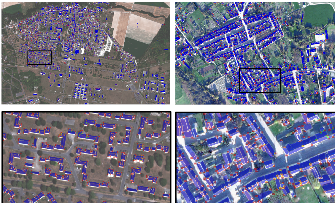
Figure 3: 3D detection of planar roof sections. KIBS detects the planar roof sections of buildings in large-scale satellite image under the form of 3D polygons. In these visual results, polygons are backprojected onto the input image (blue shapes). Red points refer to the vertices of the polygons.
