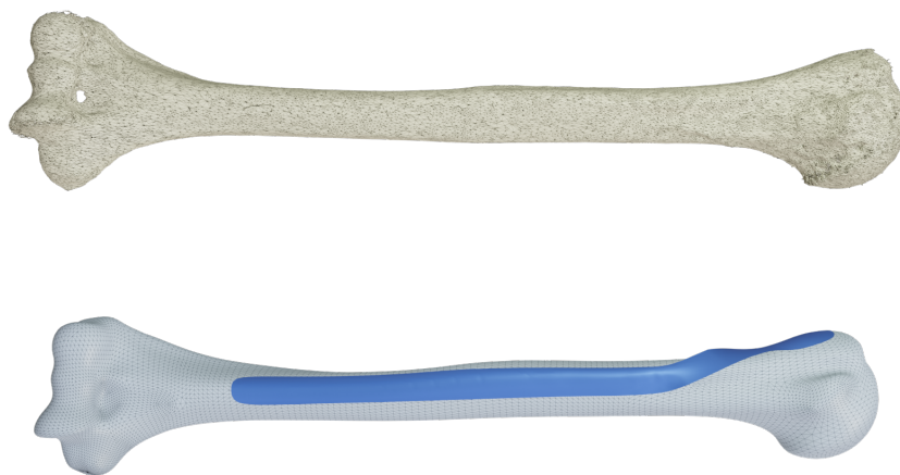
Figure 8: In this work, we investigate how to create personalized plates that match the individual shape of the bone of a patient to heal humerus fractures.
