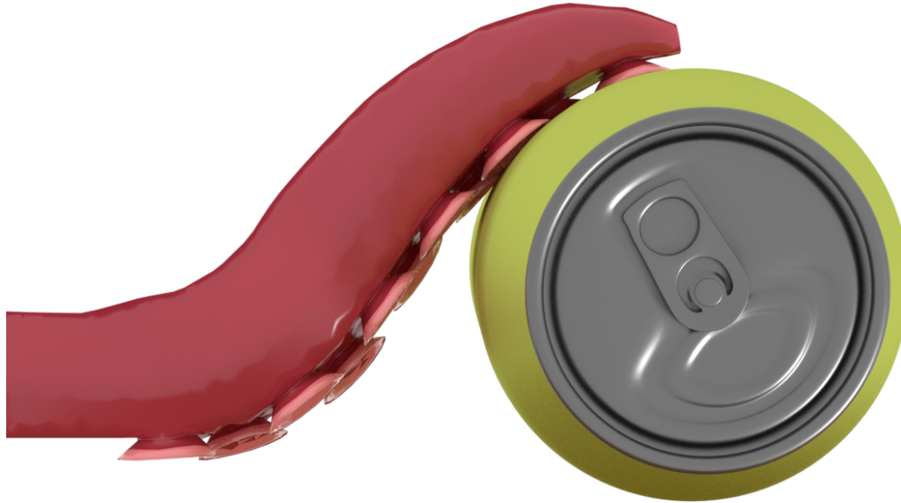
Figure 11: An octopus tentacle lifts a can using its suction cups (in simulation)
