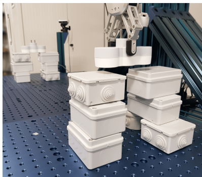
Figure 14: Example result of our approach. A UR5 manipulator assembles a configuration of known primitives (right - foreground). The configuration is specified by a single photograph of the assembly (camera on the left - background).
