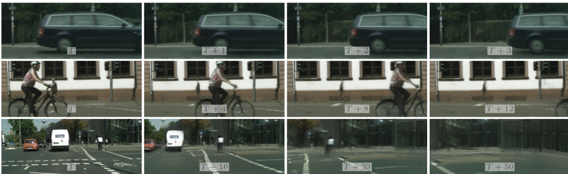
Figure 8: Video frame T and future frames T+K predicted by WALDO from frames 1 to T . In our experiments, we use in general T=4 (1/4s) and K up to 50 (3s).
