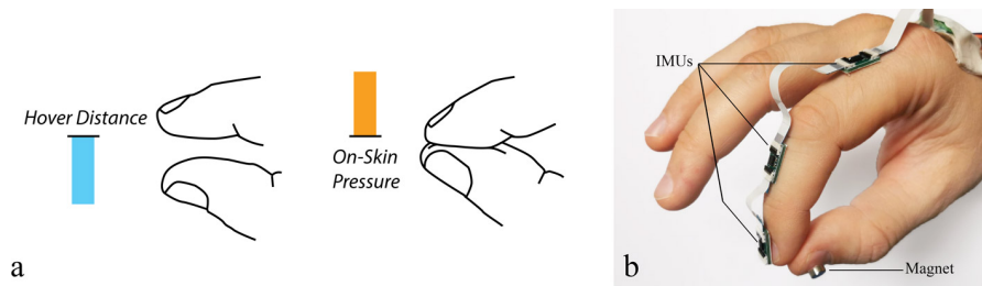
Figure 4: Magnet and IMU array system used to estimate pressure levels and hover distances between the thumb and the index finger using a BiRNN deep learning approach.
