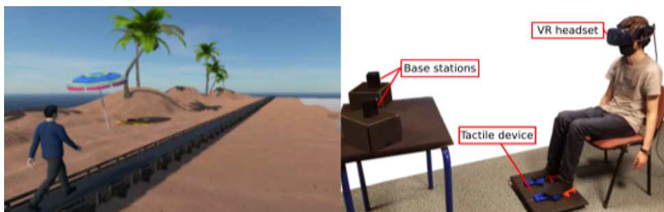
Figure 9: Experimental apparatus. Top: Virtual scene with self avatar walking. Bottom: Participant seated in a chair with feet placed above vibrotactile actuators.
