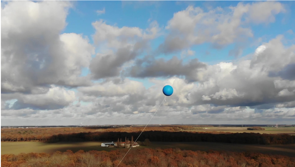
Figure 3: One of the 11 balloons used in a 103 km mesh network experiment [11]. If you look very closely, you can see the low-power wireless device hanging from the balloon.
