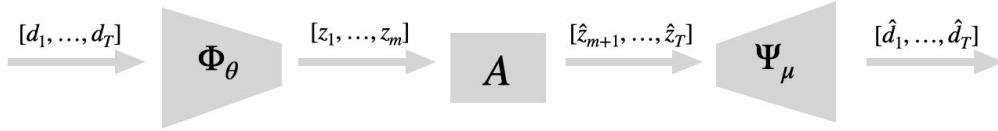
Figure 12: General overview of the proposed pipeline: the measurements [d_1, \dots, d_T] are first encoded with \Phi_\theta to codes [z_1, \dots, z_T] . Only the m first codes are used to estimate the linear system dynamics A . Using this linear dynamics A and the last code z_m , the last T - m codes are predicted. The resulting reconstructed measurements [\hat{d}_1, \dots, \hat{d}_T] are obtained by decoding with \Psi_\theta the embeddings of the actual measurements [z_1, \dots, z_m] and the predicted embeddings [z_{m+1}, \dots, z_T] .
