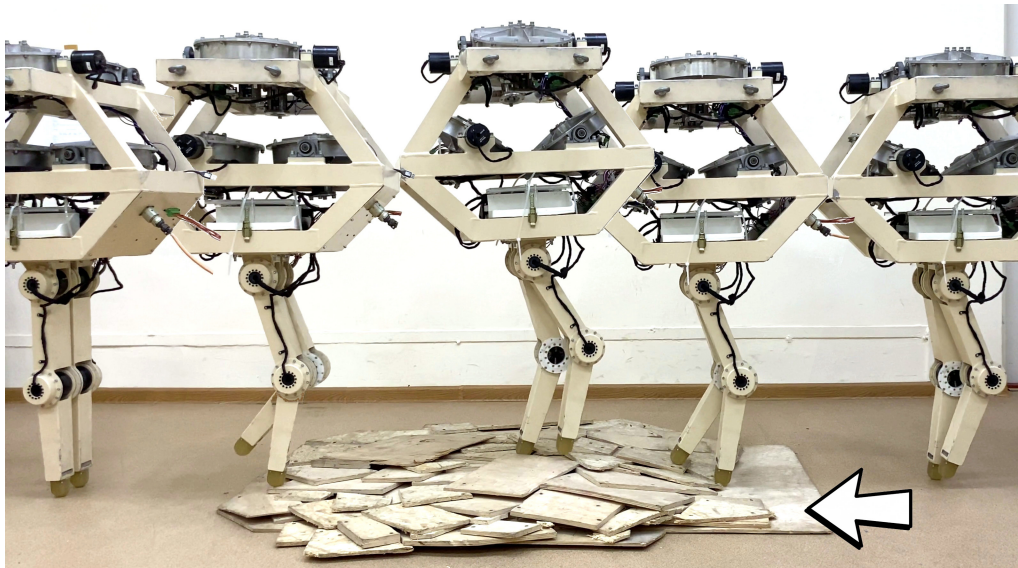
Figure 6: We are developing a biped that uses four control moment gyroscopes as an auxiliary stabilization system.
