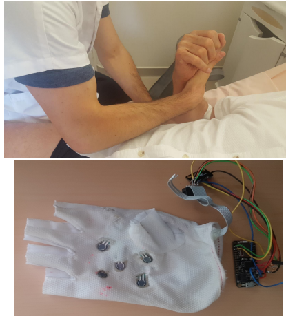
Figure 2: From left to right: a motricity test, the glove with the 5 force sensors, the ARM processor and the accelerometer
