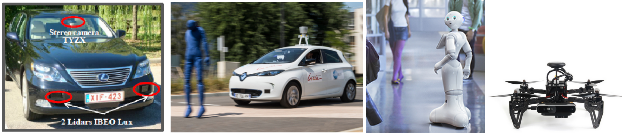
Figure 2: Most of the Chroma platforms: the equipped Toyota Lexus, the autonomous version of the Renault Zoe car, the Pepper humanoid, the PX4-Vision UAV.
