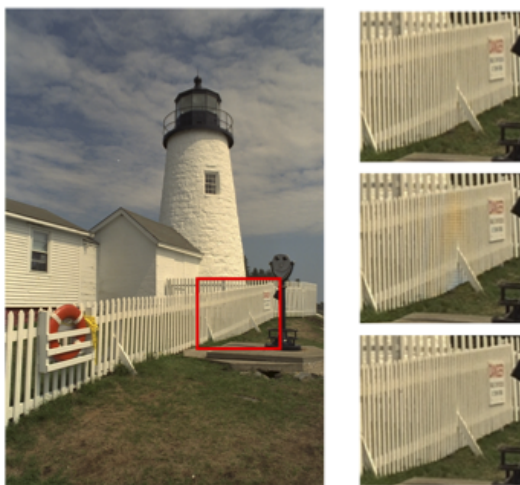
Figure 7: Demosaicking result obtained by our method. Top right: Ground truth. Middle: Image demosaicked with our sparse coding baseline without non-local prior. Bottom: demosaicking with sparse coding and non-local prior. The reconstruction does not exhibit any artefact on this image which is notoriously difficult for demosaicking.
