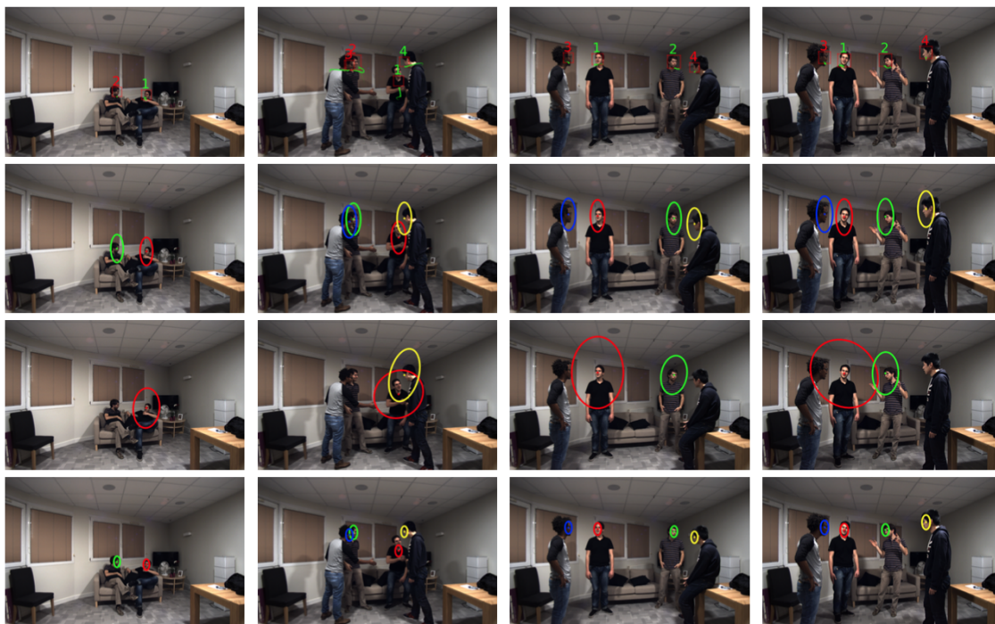
Figure 1: This figure illustrates the audio-visual multiple-person tracking that has been developed by the team [43, 30]. The tracker is based on variational inference [5] and on supervised sound-source localization [11, 34]. Each person is identified with a digit. Green digits denote speaking persons, while red digits denote silent ones. The next rows show the covariances (uncertainties) associated with the visual (second row), audio (third row) and dynamic (fourth row) contributions for tracking a varying number of persons. Notice the large uncertainty associated with audio and the small uncertainty associated with the dynamics of the tracker. In the light of this example, one may notice the complementary roles played by vision and audio: vision data are more accurate while audio data provide speech information (who speaks when). These developments have been supported by the European Union via the FP7 STREP project “ Embodied Audition for Robots ” (EARS), the ERC advanced grant “ Vision and Hearing in Action ” (VHIA) and ERC Proof of Concept grand VHIALab.
