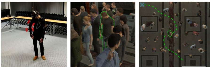
Figure 16: Our objective is to understand whether and to what extent providing haptic rendering of collisions during navigation through a virtual crowd (right) makes users behave more realistically. Whenever a collision occurs (center), armbands worn on the arms locally vibrate to render this contact (left). We carried out an experiment with 23 participants, testing both subjective and objective metrics regarding the users' path planning, body motion, kinetic energy, presence, and embodiment.
