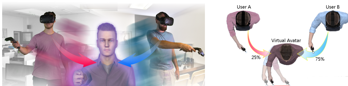
Figure 12: Our “Virtual Co-Embodiment” experience enables a pair of users to be embodied simultaneously in the same virtual avatar (Left). The positions and orientations of the two users are applied to the virtual body of the avatar based on a weighted average, e.g., “User A” with 25% control and “User B” with 75% control over the virtual body (Right).
