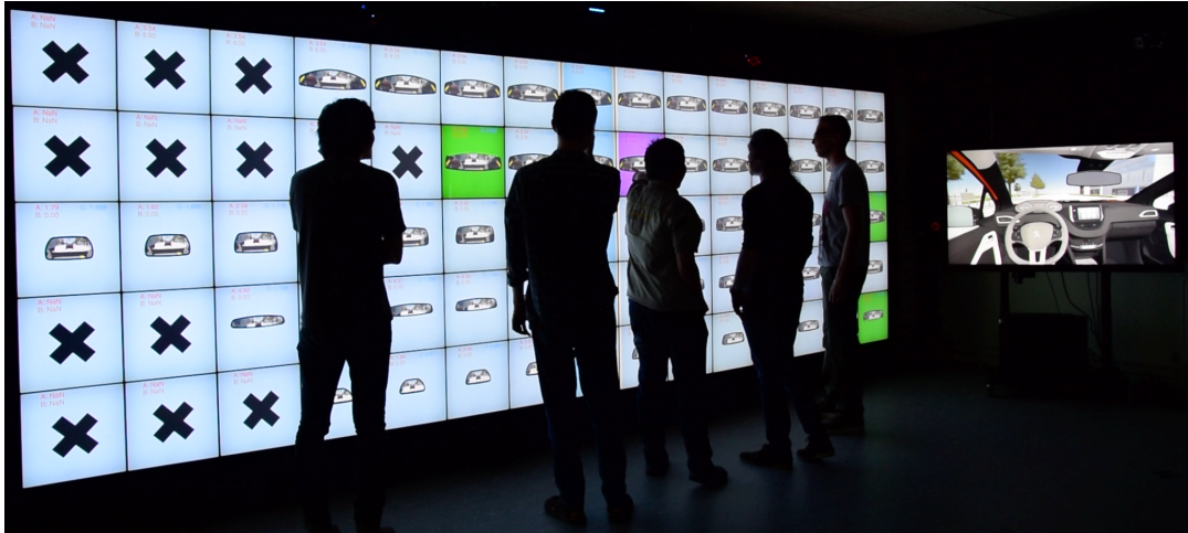
Figure 4: ShapeCompare [25] enables non-CAD experts to generate and explore multiple design alternatives on a wall-sized display.
