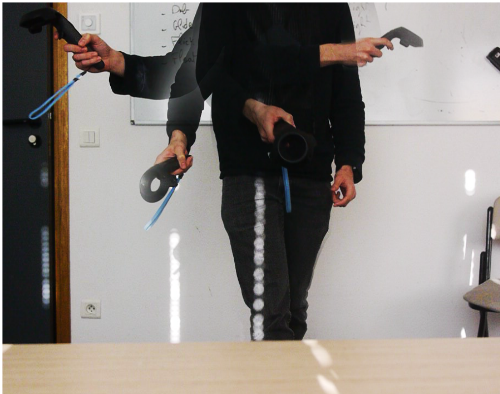
Figure 4: We compute Laban effort qualities from the rigid motion of virtual reality trackers and use them in computer puppetry applications.
