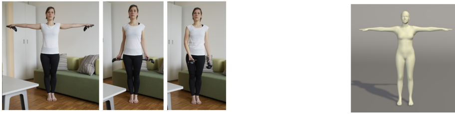
Figure 5. Using the wand controllers of the HTC Vive, the Virtual Caliper produces a rigged 3D model with exactly the dimensions of the measured person.
