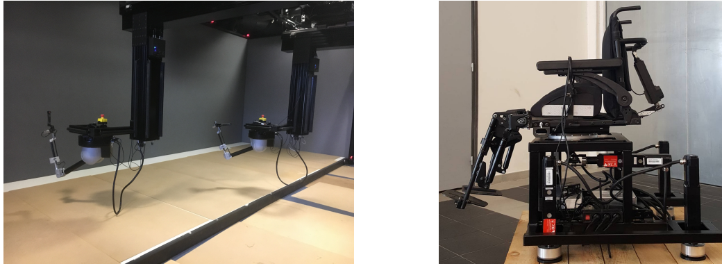
Figure 2. Immersia platform: (Left) “Scale-One” Haptic system for one or two users. (Right) Motion platform for a powered wheelchair simulation.
