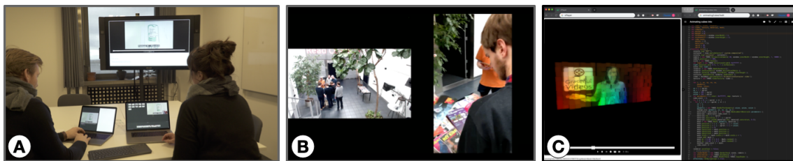
Figure 3. Videostrates examples: A) Two users collaboratively edit the same videostrate , one with a timeline-based editor and the other with a subtitle editor. The results appear in a live, interactive preview on a large screen. B) Videostrates aggregates, broadcasts and records multiple live streams, here from a statically mounted camera and a smartphone. C) A Videostrate -based computational notebook uses Codestrates to programmatically create a WebGL animation and synchronize its playback with recorded video composited with a green screen.
