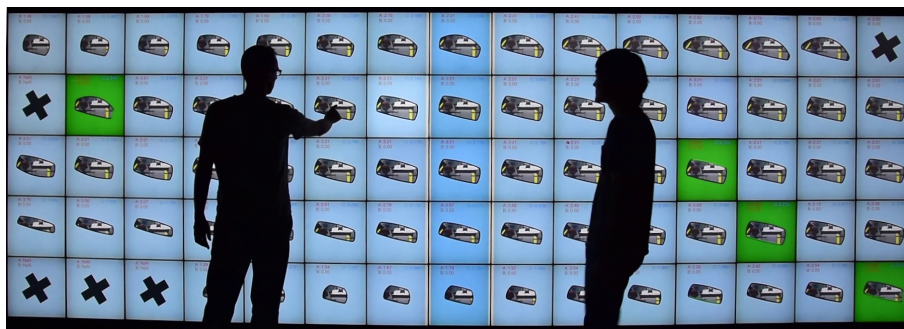
Figure 4. Collaborative exploration of multiple design alternatives of a car rear-view mirror on a wall-sized display.
